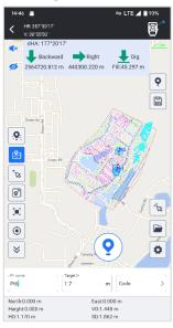
CAD Stakeout allows you to import **CAD basemap** and stakeout it, without inputting point coordinates one by one.
