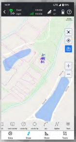
This feature enables CAD drawing capabilities, which were previously only possible on a PC. Now surveyors can edit CAD map on RTK controller or tablet or phones.
